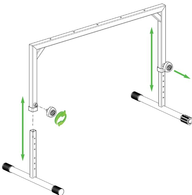
Screw spring-loaded clamping knobs into the U-frame with approx. five turns. Slide the base frame into the U-frame. Make sure that the holes in the base frame point in the direction of the locking screw. Tightening the spring-loaded clamping knobs to fix the height of the base frame.
