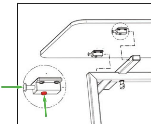
To place the tabletop, the four quick-release clamps must be "opened", by pressing the red button on the quick-release clamps. The locking pin snaps back and the tabletop can be mounted or dismounted. Place the tabletop on the support tubes and secure it with the support tubes by pressing the locking pins. Make sure that the locking pins are inserted into the holes and bolted.
