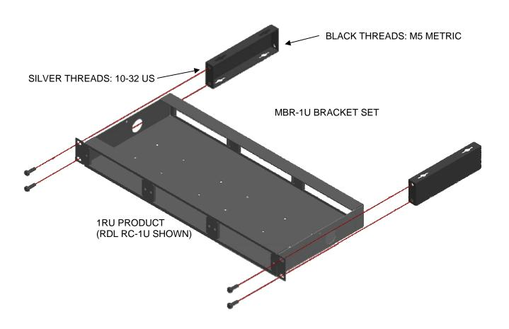
Mount brackets to table or under counter with either US or metric threads facing forward. Secure any 1 RU product to the brackets.
